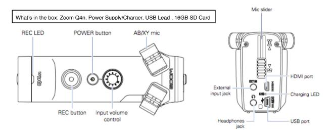
The Zoom Q4n is a HD quality video/audio recorder with variable gain and mic positioning. Mic position is changed by sliding the rear slider up/down, then manually adjusting the mic capsules to position Here are the basic operation instructions:
