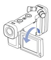
1. Rotate the screen in the direction of the arrow.
