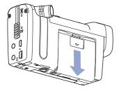
1. Slide the **Q4** battery cover down to remove it.
